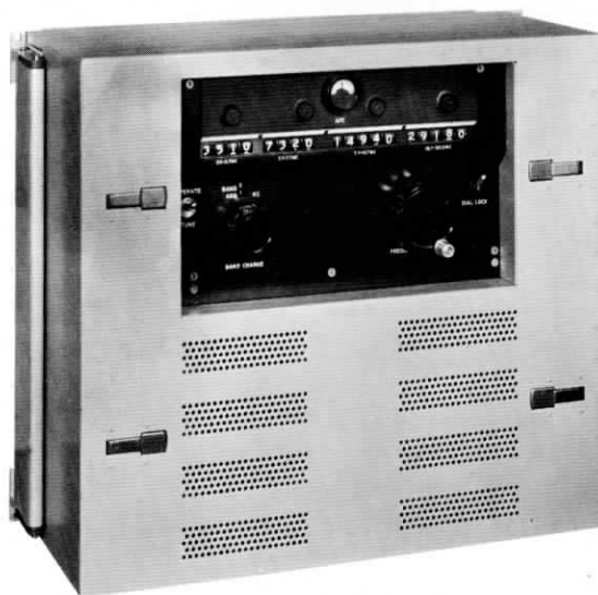
Figure 1. Frequency Generator 786E-1 translates intermediate frequencies to r-f or radio frequencies to i-f
