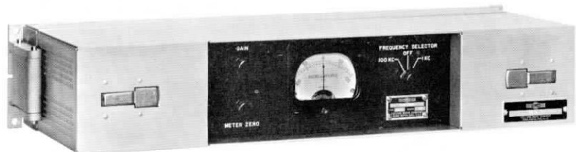
Figure 28. Frequency Comparator 54Q-1 compares reference oscillator signal with external standard.
