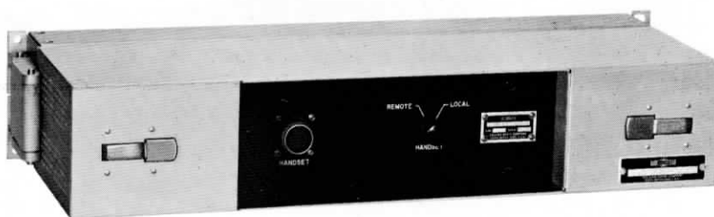
Figure 32. Collins Handset Adapter permits local or remote receiver operation
