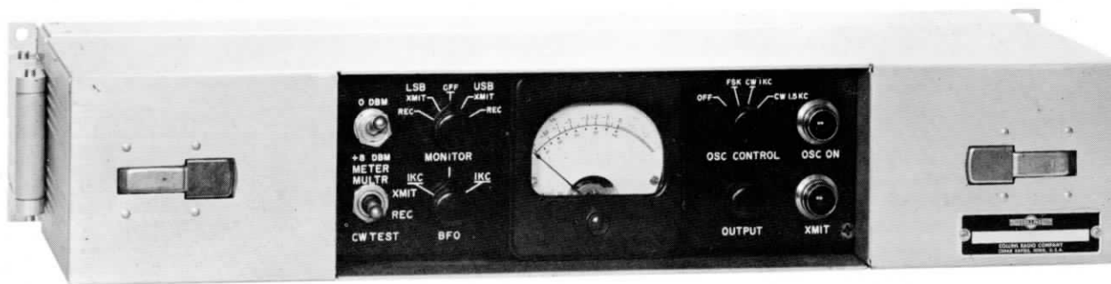
Figure 35. CW and FSK Unit also monitors the receive and transmit audio outputs of the audio and control units
