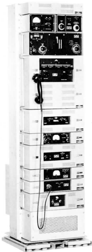
Figure 47. Another typical pattern (Column D) is the KWT-6 Type 8 transceiver with power amplifier and other units
